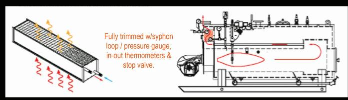
"One could think of this as a built in feedwater heater, ensuring that the make-up water used to replenish the boiler is pre-heated to near boiling temperatures."
